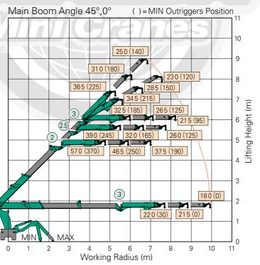
The values in are rated total load (kg), they are based on the actual working radius including boom & jib deflection.
